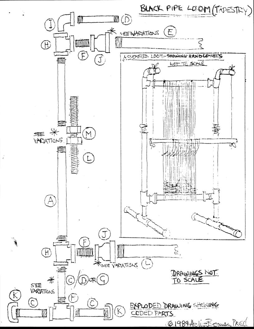
CONSTRUCTING A FREE STANDING TAPESTRY LOOM, using standard black pipe plumbing parts, and offering a four feet wide weaving width. Dimensions are approx. 7 ft. x 4 1/2 ft. x 3 ft.
